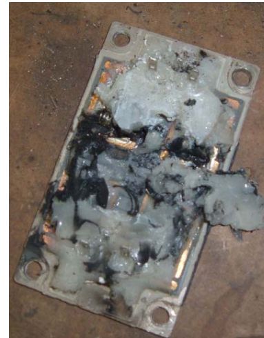
Picture 3: Consequence of IGBT transistor explosion
