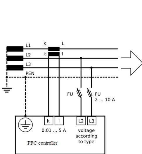
Picture 3: Connection of measuring circuits
