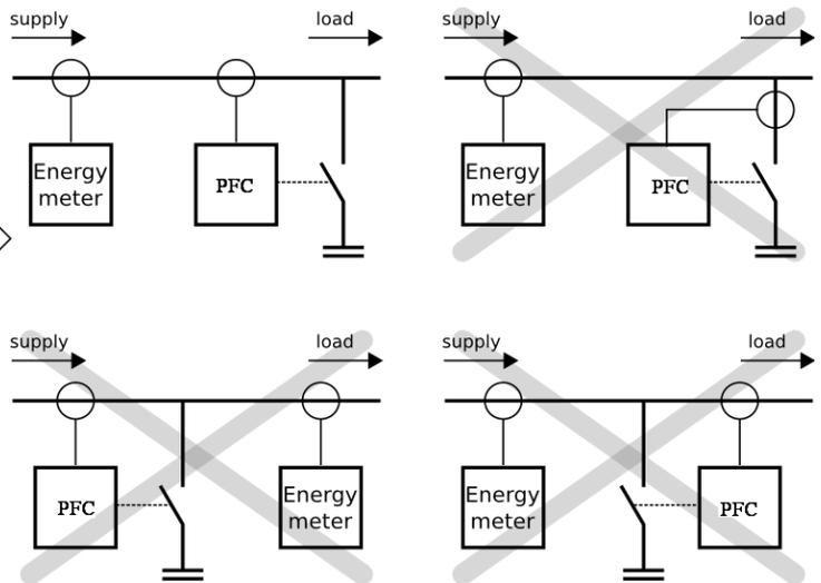
Picture 4: Position of PFC controller in the system
