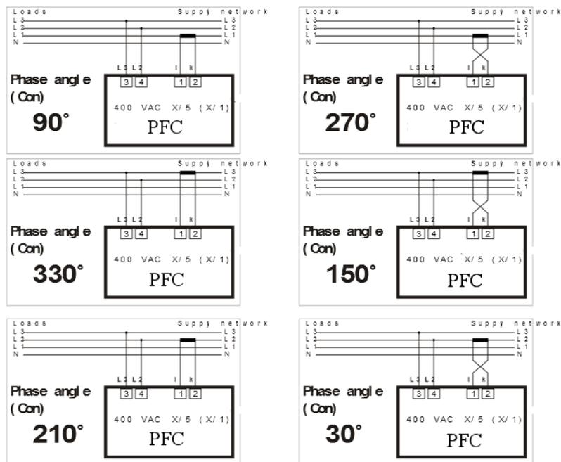
Table 6. Phase shift setting for supply and measuring voltage 400 VAC
