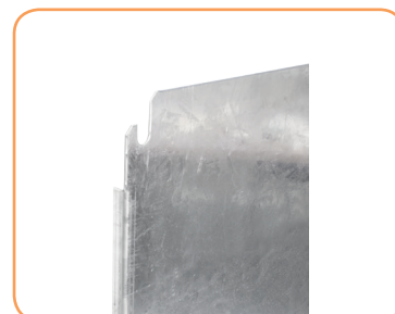
Mounting plate is made of galvanized steel sheet with a thickness of 2 mm. Mounting plate is fixed to the body with screws M8x25 mm. Depending on the size, special foldings of the plate edge are made for better stiffness.
