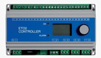
ETO2 is controller for ice and snow melting on the ground and in gutters. Using readings from temperature and moisture sensors, the controller ensures economical control of power consumption while keeping outdoor areas and roofs free of ice and snow. The moisture sensor should be installed in the ground surface or placed in the gutter. As soon as moisture is detected in conjunction with low temperature, the ETO2 controller activates the snow-melting system.
