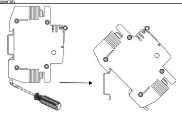
Using a screwdriver pull down on the plastic snap-on unit.
