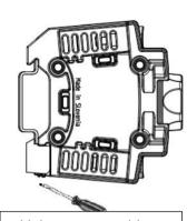
Using a screwdriver pull down on the plastic snap-on unit
