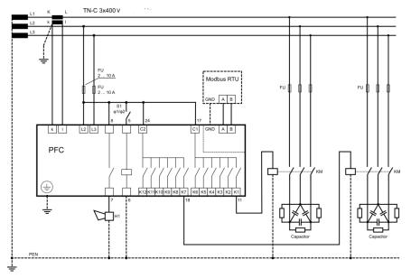
Picture 5: Connection of the PFC 12 for standard supply voltage 400 VAC
