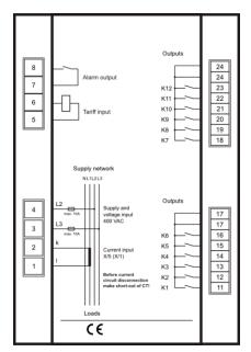
Picture 2. Device terminal connection
