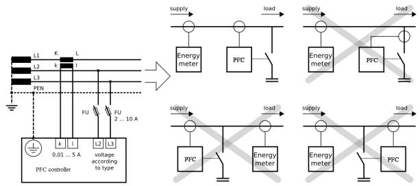
Picture 3: Connection of measuring circuits
