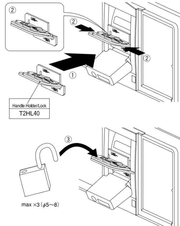
•Handle holder/ lock can be fitted in any position of | (ON) and ○(OFF).
