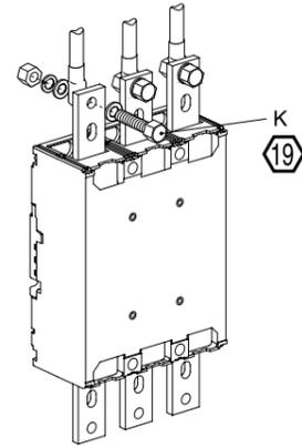
•Insulate all bare conductors of the line side until the breaker end.
